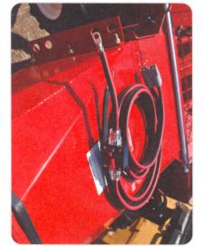
Step 9 Cut tractor harness to proper length to reach tractor battery.
