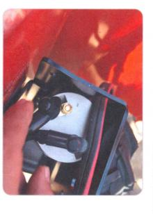
motor and control box. Attach longer leg of Y-Step 7 Install drive motor Y-harness between drive on the Y harness and control box) harness to the bottom studs on control box (\*Mover direction can be reversed by reversing wires
