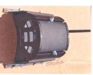
Step 2 Installing control box bracket Install control box bracket using 1/4 x 3/4 bolt and
