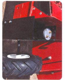
mounting plate by using 3/8" x 9" bolt and Step 5 Install drive motor assembly to the
