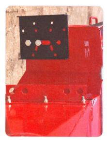
using existing holes Step 4 Bolt both mounting brackets onto auger
