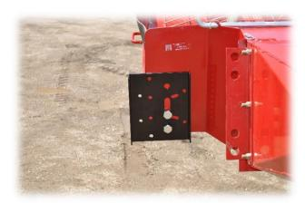
**Step 4-** Bolt both mounting brackets onto auger using existing holes.
