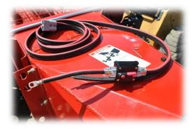
**Step 9**- Cut the tractor harness to the proper length to reach the tractor battery. Install the circuit breaker as close to the positive battery post as possible. Be sure you have 12 volt operating system on your tractor.
