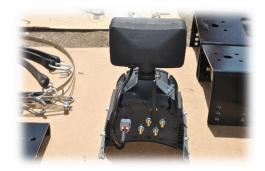
Note the secured light that is plugged firmly into the back of the control box. Note the secured control box brackets on the side.
