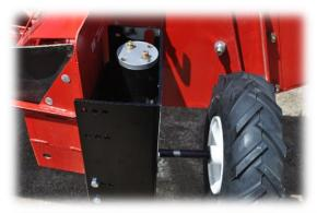
**Step 5-** Install drive motor assembly to the mounting plate by using 3/8" x 9" bolt and locknuts. Achieve desired height by sliding the bracket up or down selecting appropriate
